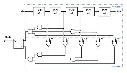
• Add 'S' Detector to control the 'Mode' signal.
