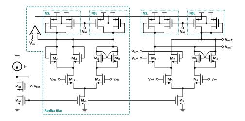
• With BPC technique, self-resonate frequency of prescalers can be fixed, and so we can dramatically decrease the power consumption of prescaler.
