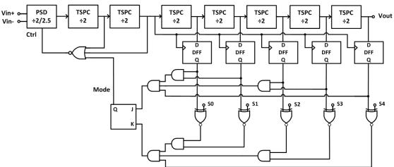
• Modulus=P\*8+S\*(0.5), for 5-bit P-counter and P/S Detector.  $\rightarrow$  Modulus= 256.5~271.5 (in steps of 0.5)
