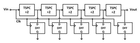
• Use D Flip-flop to match the signal to avoid glitch.
